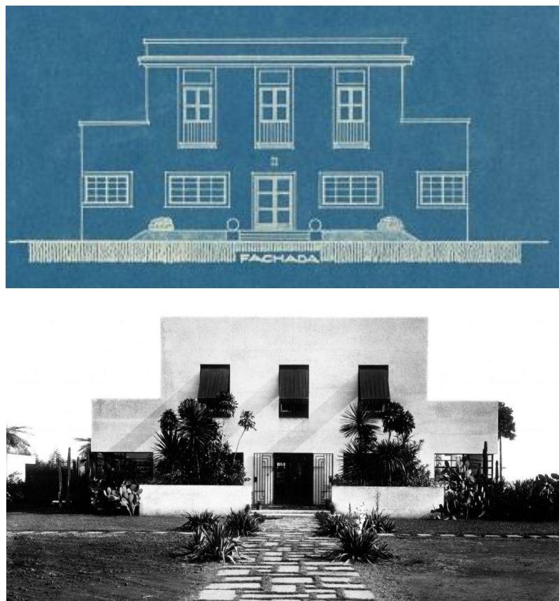
Figure 21 - Gregori Warchavchik, House at Santa Cruz Street (1928). (Top) Façade submitted to the Municipality / (Bottom) Built façade.
