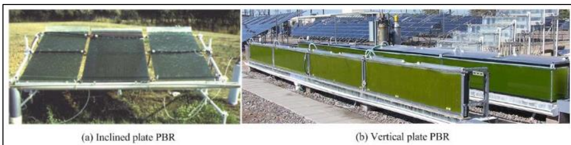
Figure 5. Flat plate photobioreactors designs Source: SHEN et al. (2009).
