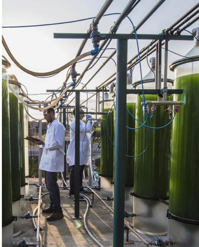
Figure 52. Microalgae cultivation in PBRs in the pre-industrial scale pilot plant Source: InterCement (2017).
